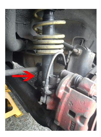
Once you've got the wheel off, the drop link is located behind the shocker, indicated by the red arrow in the picture above.
