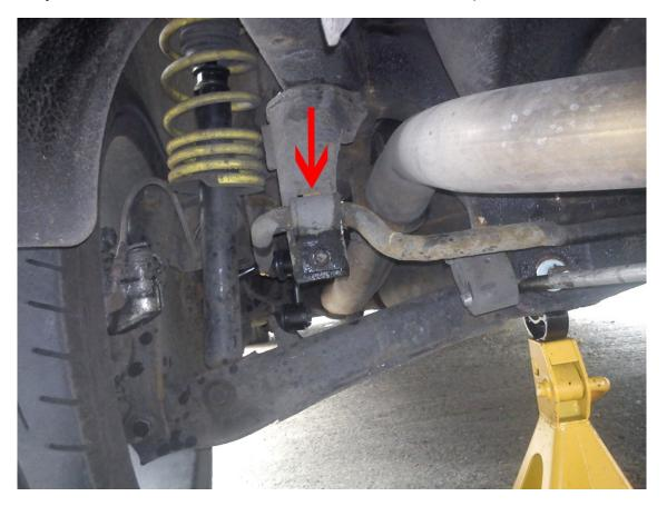
Here's a closer picture of the bush and the clip holding it in place, which is secured by a 12mm bolt, indicated by the red arrow.
