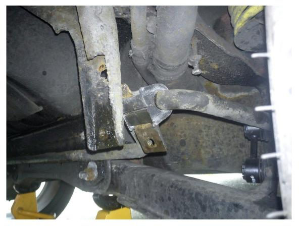
The above picture is actually of the off side ARB bush, which is mounted the other way round to the near side. You can see the hole the clip's lug fits in to. Getting the lug in to this hole can be a bit tricky, but if your drop links have not siezed, there should be a fair bit of movement to allow you to manouvere it in.
