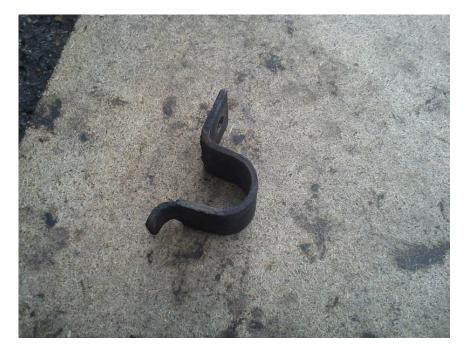
The top of the clip, is secured with a lug sliding in to a hole and then held in place with the 12mm bolt at the bottom. Removing the bush is very simple as it has a split at its base, alowing it to be pushed over the ARB.
