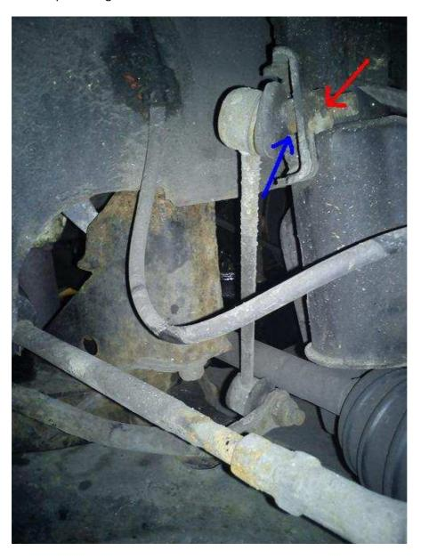
Next you need to loosen the 17mm nuts, starting here with the lower one. Put the 14mm spanner behind the ARB and your 17mm spanner on the front nut, you can position the 14mm spanner so it leans against the strut and will stop the ball joint spinning inside the drop link .
