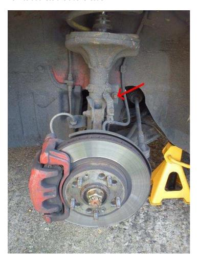
Once you've got the wheel off, the drop link is located behind the strut, indicated by the red arrow.
