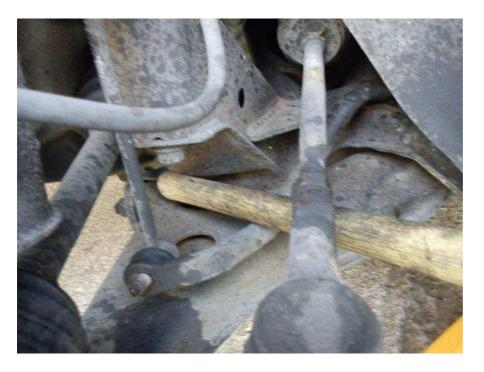
Next repeat the previous step to loosen and remove the upper bolt and then remove the drop link
